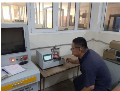
2-rasm. Bitumni yumshash haroratini "Xalqa va shar" usulida sinash
