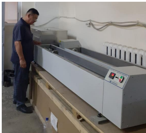
3-rasm. Bitumni cho'ziluvchanligini duktometr asbobida sinash jarayoni
