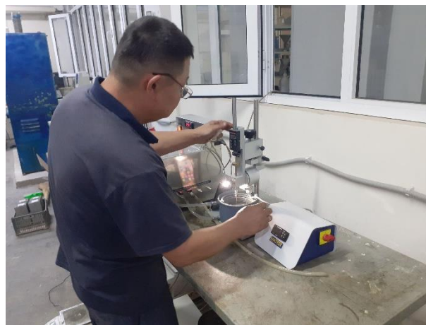
1-rasm. Bitumning penetratsiyasini Penetrometr asbobida sinash jarayoni
